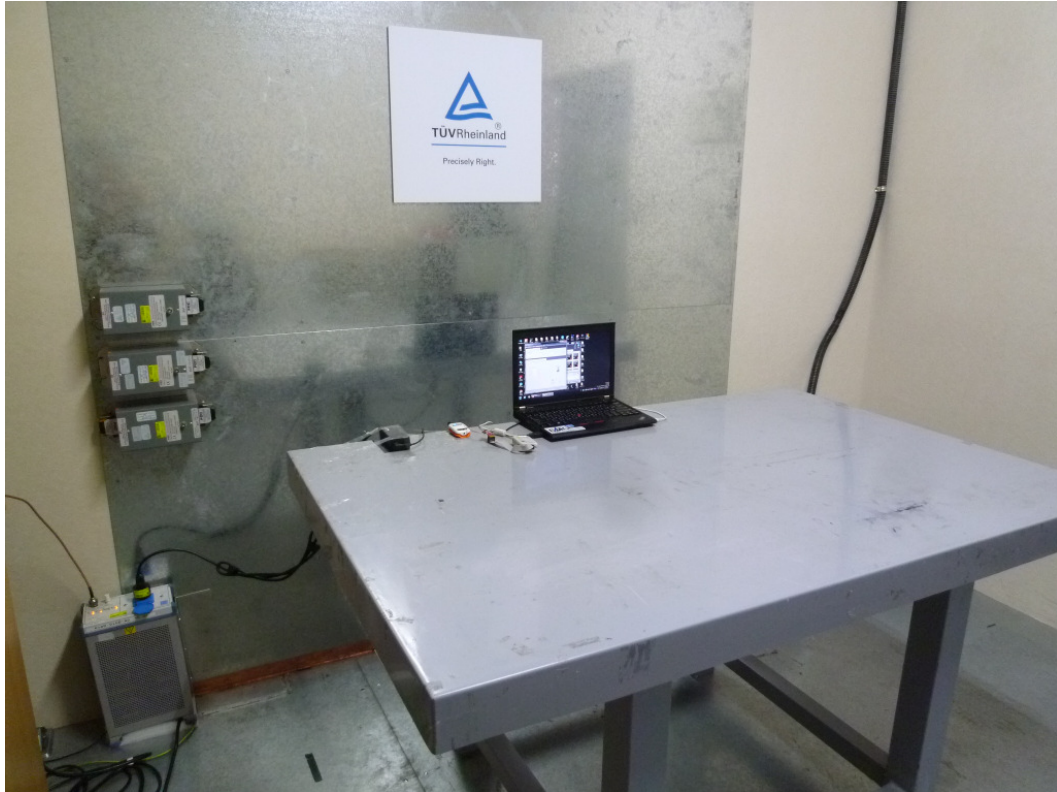
Photograph 6: Set-up for Mains (Front View)
