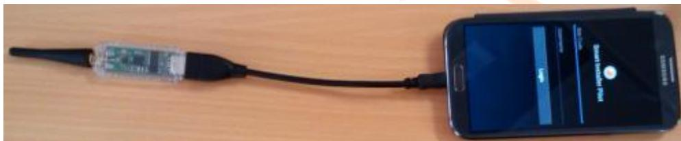
The dongle connects to the Smartphone via the mini-USB port. Once connected, the LED on the dongle should flash and the Smartphone will state that a USB device is connected.
