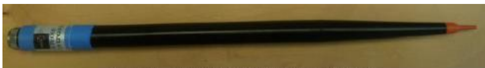
Figure 1 – MVG COMOSAR Dosimetric E-field Dipole
