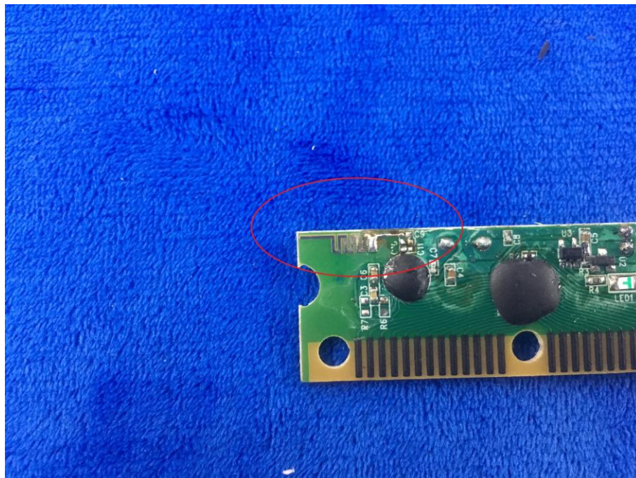
Antenna View (RX)
