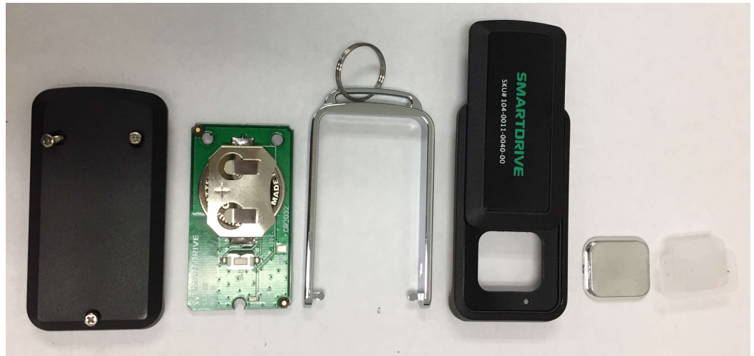
Internal Exploded View, Bottom PCB
