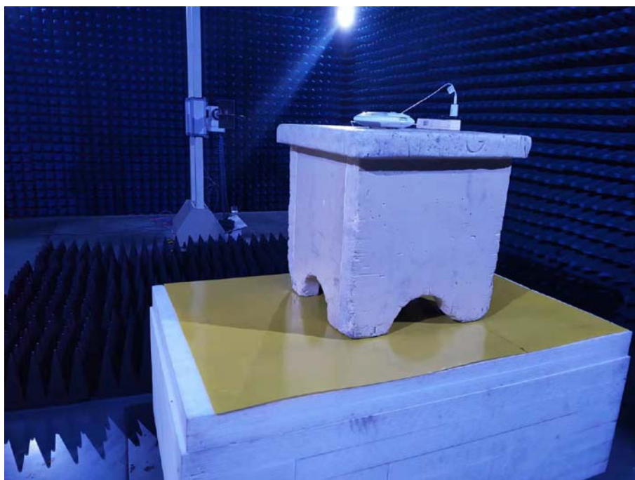
Photo of Radiated Emission Measurement Above 1GHz
