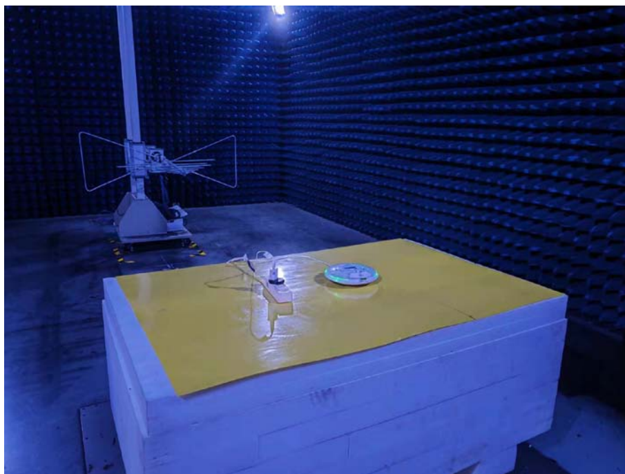
Photo of Radiated Emission Measurement Below 1GHz
