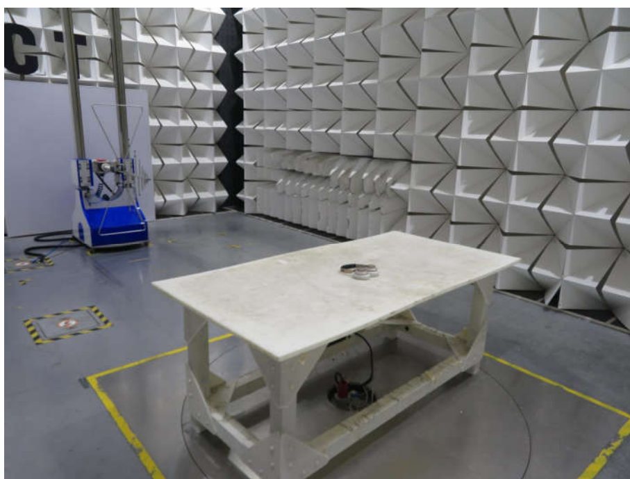
Radiated spurious emission Test Setup-2(Below 1GHz)
