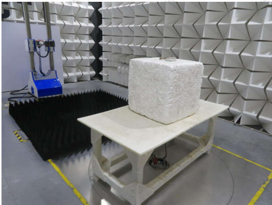
Radiated spurious emission Test Setup-3(Above 1GHz)
