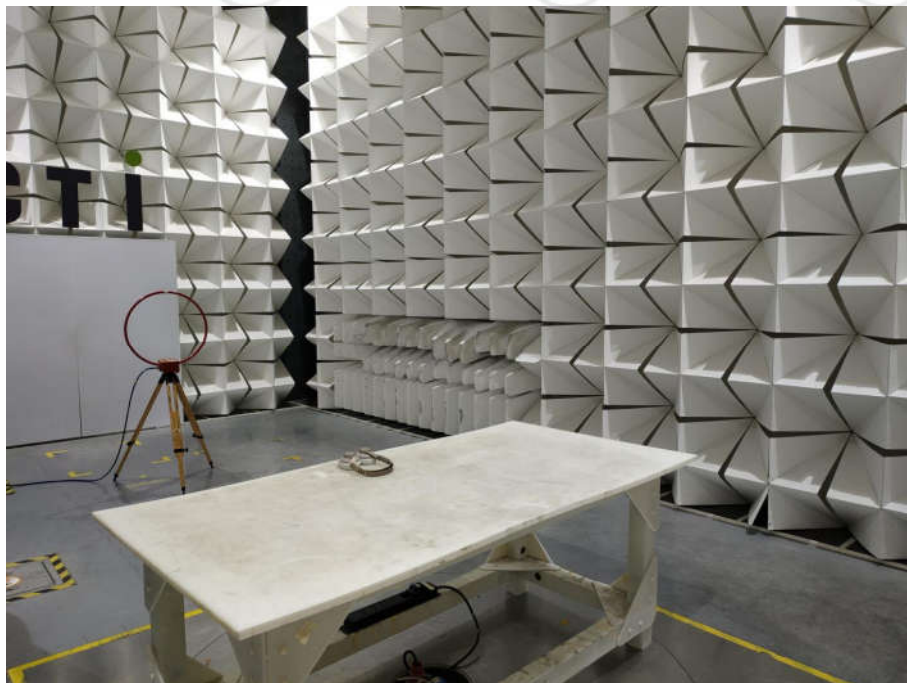
Radiated spurious emission Test Setup-1(Below 30M)
