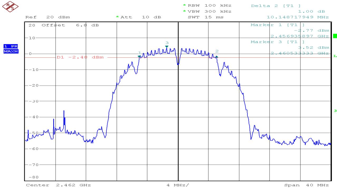
**IEEE 802.11g MODE /Chain 0****6dB Bandwidth (CH Low)**
