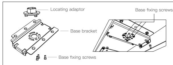
2. Install the device on the locating adaptor; fasten screws after adjusting the horizontal angle. Remove the cover from the device holder to adjust angle, then release elevation locking screws; fasten screws while completing angle adjustment.
