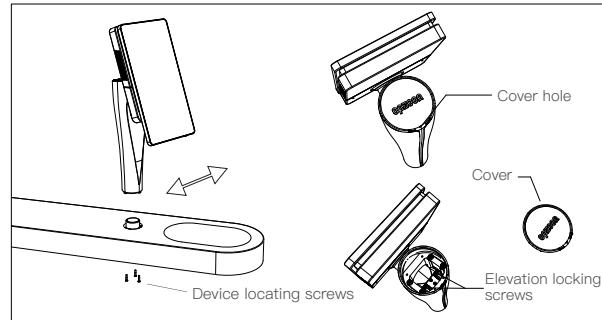
3. Install the interface module to the reserved mounting location under the gate cover.
