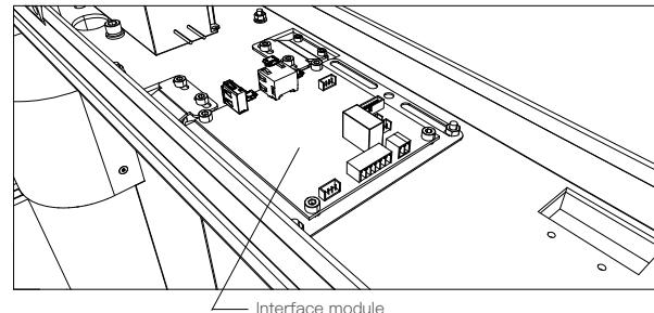
4. Connect cables to the interface module, and then cover the gate cover.
