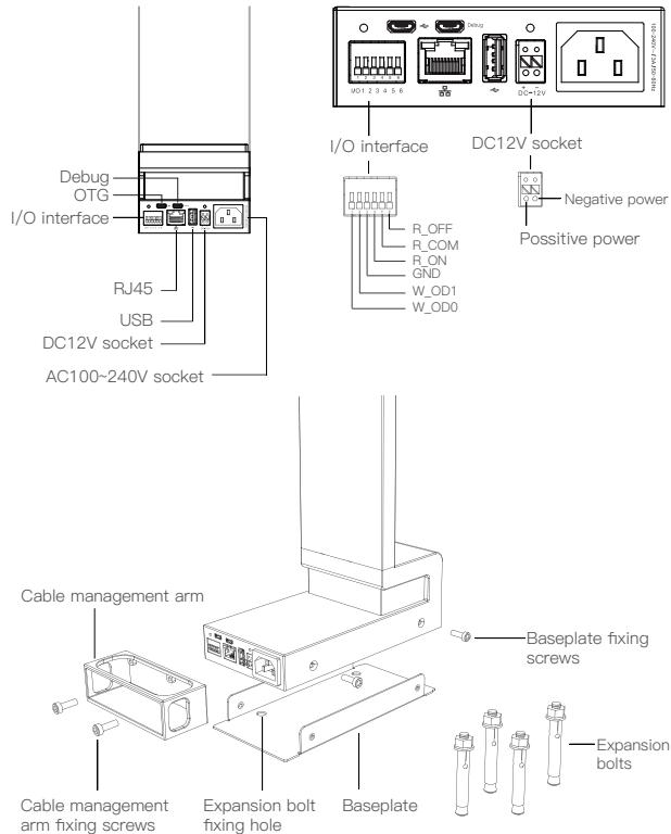
1. While installing gates, first remove the four flat-head hexagon screws on the side of the base and remove the baseplate.
