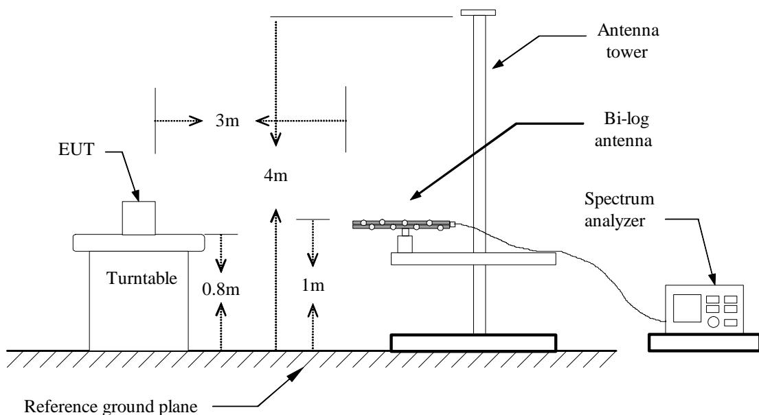
**Above 1 GHz**
