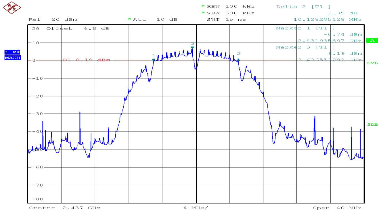
**6dB Bandwidth (CH High)**
