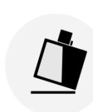
**Safety Interlock in Protective Housing:** The shield is a protective housing which prevents users access to laser radiation in excess of the AEL for Class 1. In addition, a micro switch attached at the bottom of the shield as a safety interlock is provided to prevent the protective housing from accidental displacement or removal.
