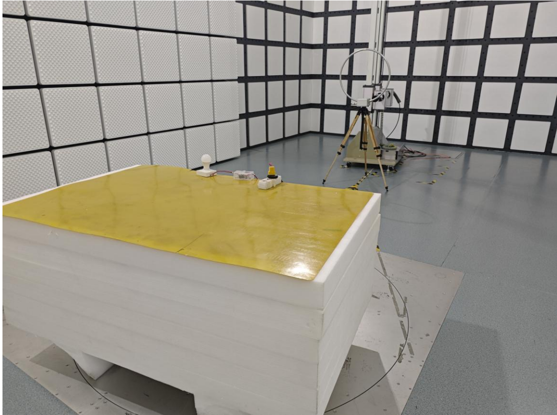
Radiated Spurious Emissions Test View (9kHz-30MHz)
