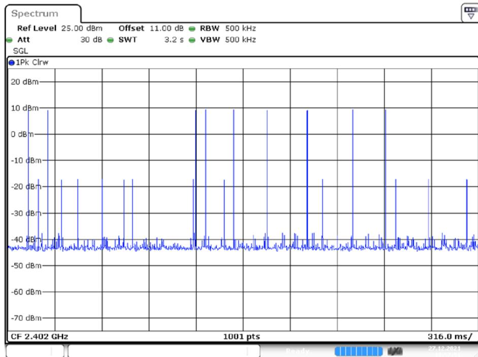
**EDR Mode ( $\pi/4$ -DQPSK)****2DH1: Pulse Width**
