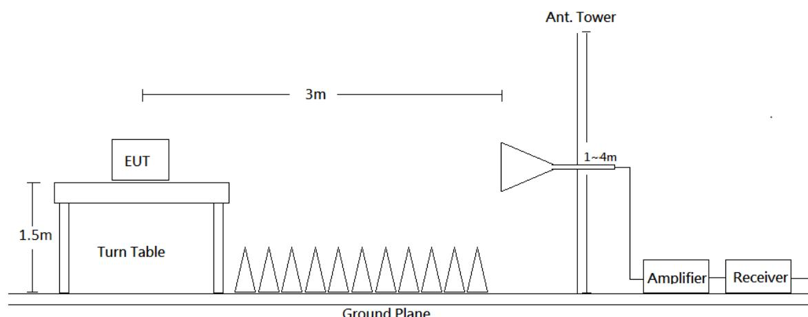
Radiated emission tests were performed in the 3 meters chamber test site, using the setup accordance with the ANSI C63.10-2013. The specification used was the FCC Part 15.209 and FCC 15.247 Limits.
