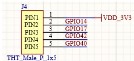
5p is equipped with a 2.54mm spacing busbar interface, and internal wiring is connected to GPIO14, GPIO17, GPIO42, GPIO40, and 3.3V.
