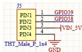
The 4p is configured with 2.54mm spacing bus ports, and the internal cables are GPIO38, GPIO39, 5V, and GND.
