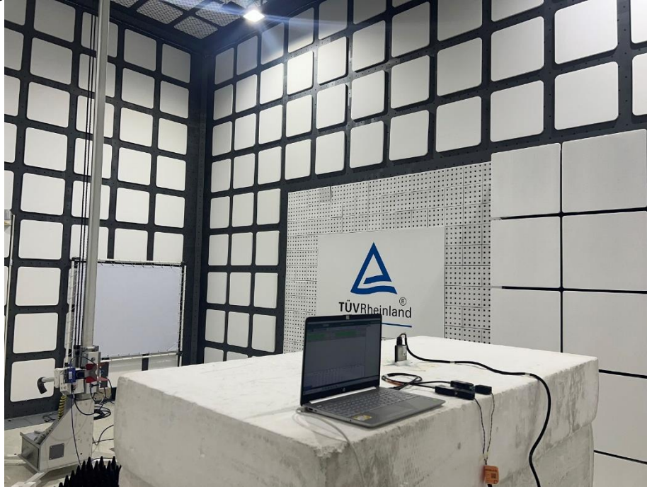
Photograph 6: Test Setup for Spurious Emissions (Back View 4)
