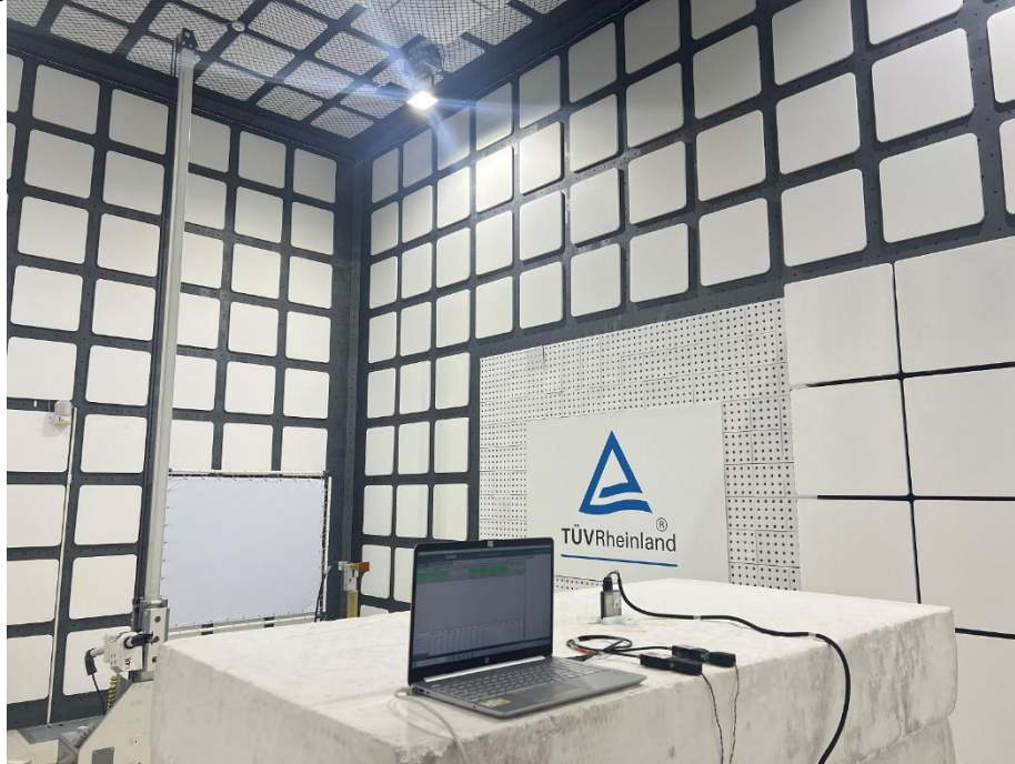
Photograph 8: Test Setup for Spurious Emissions (Back View 6)
