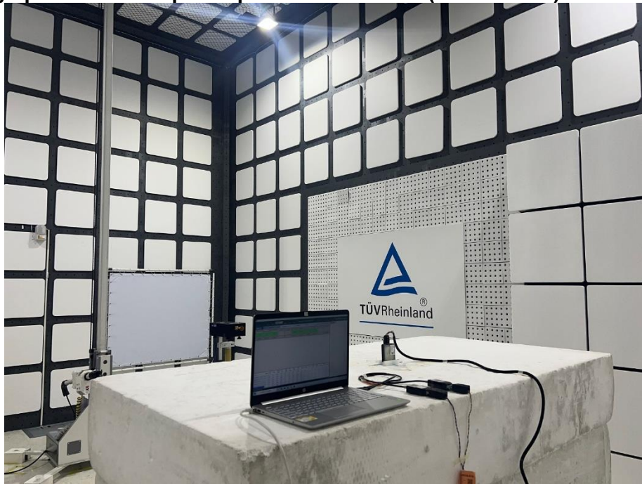
Photograph 8: Test Setup for Spurious Emissions (Back View 6)
