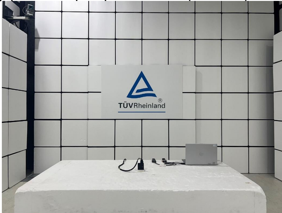
Photograph 2: Test Setup for Spurious Emissions (Front View 2)
