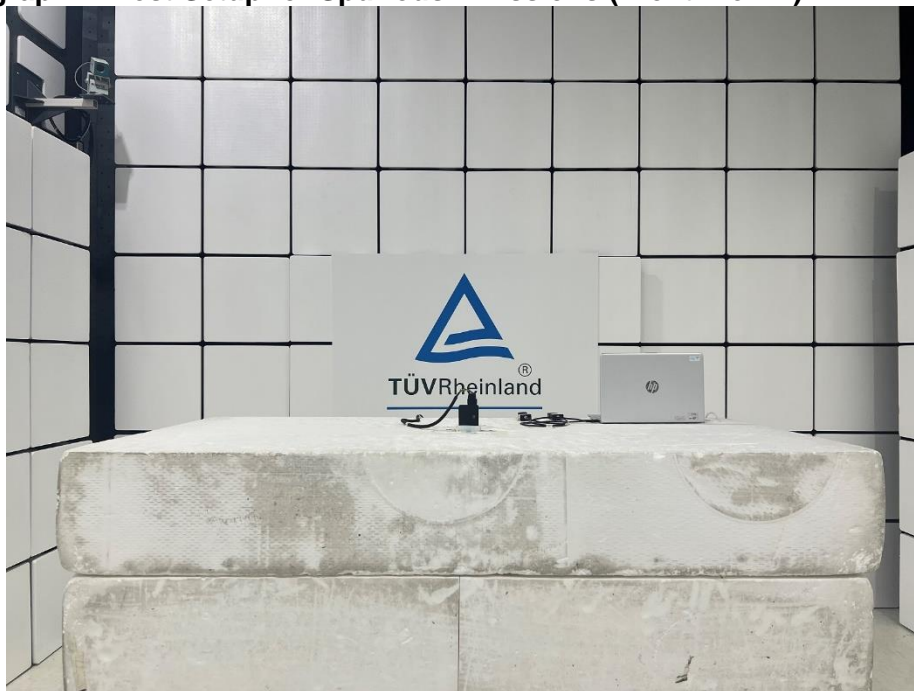
Photograph 2: Test Setup for Spurious Emissions (Front View 2)
