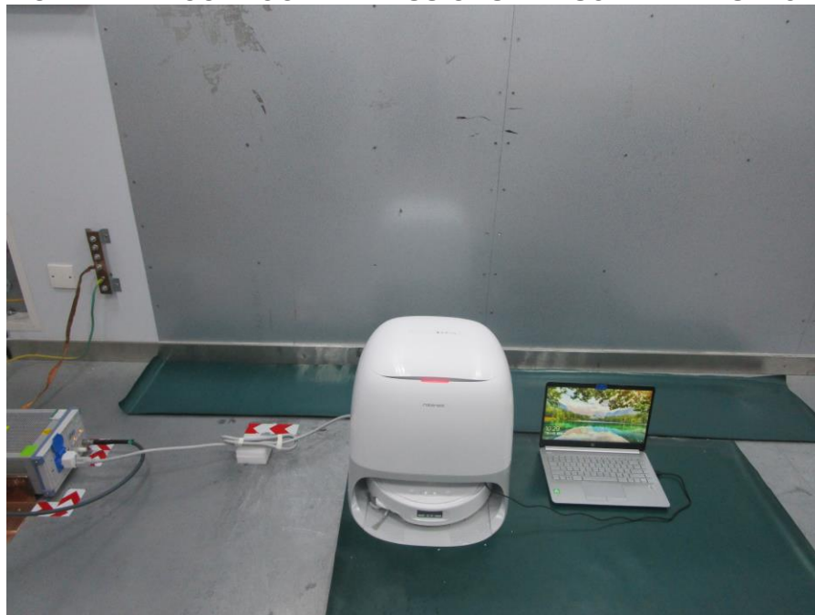
POWERLINE CONDUCTED EMISSIONS MEASUREMENT SETUP
