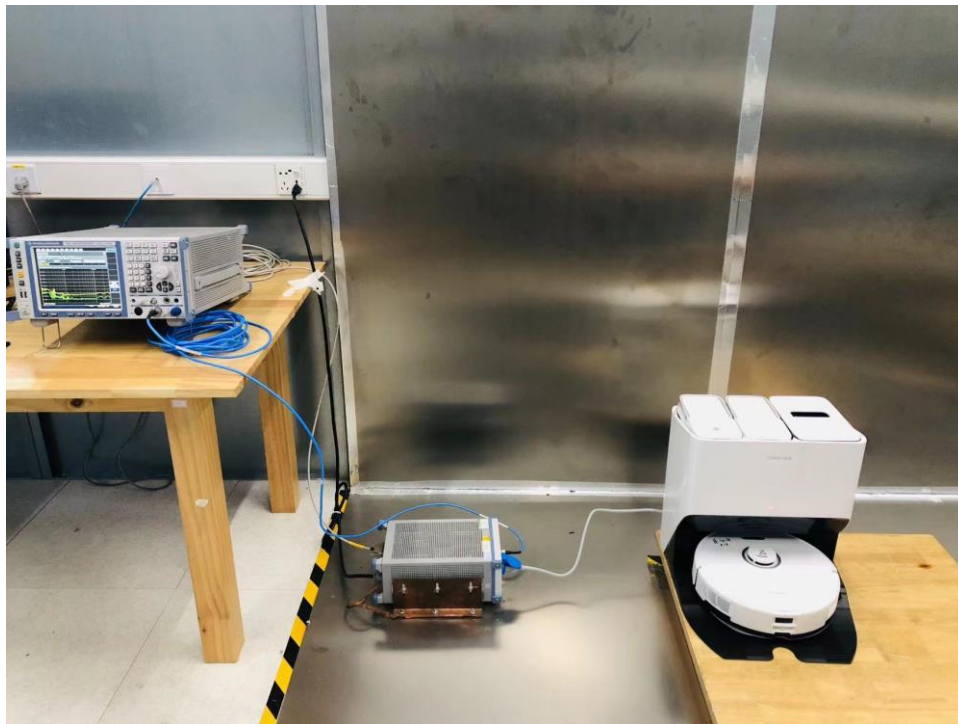
Photograph 3: Set-up photo for Conducted Emission
