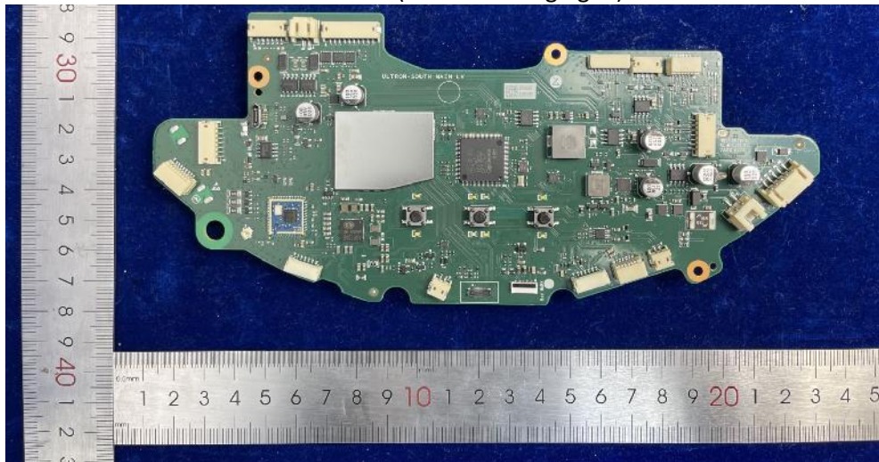
Main board (use new charging IC)
