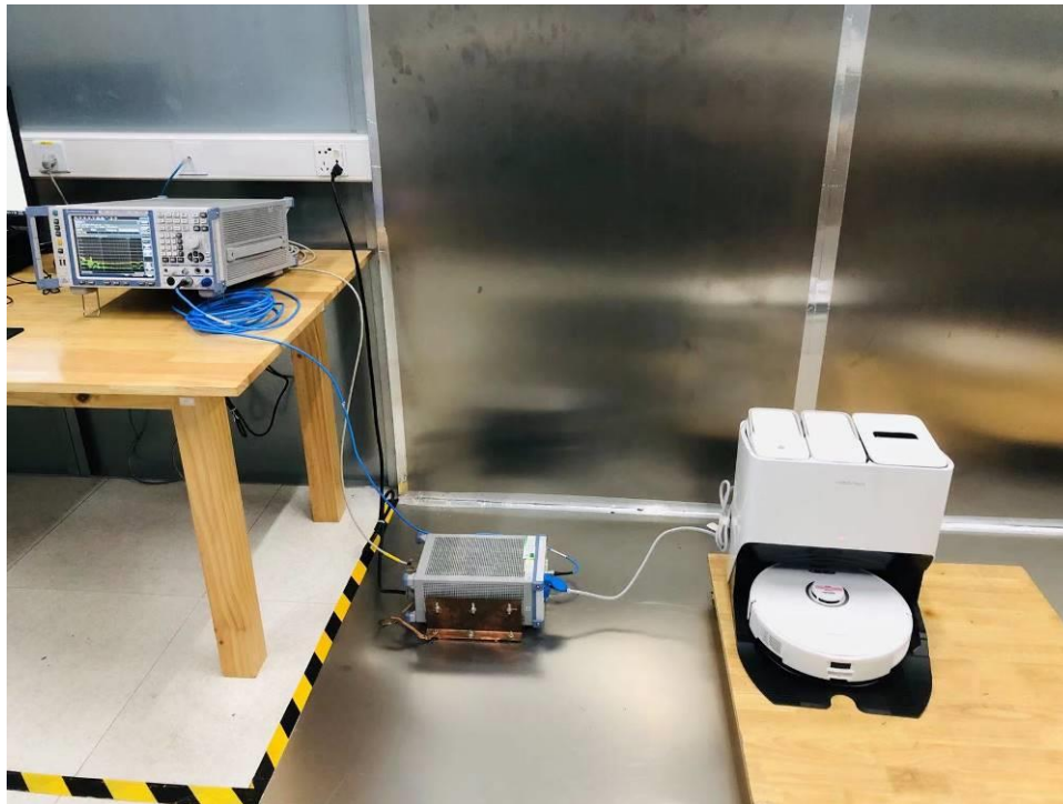
Photograph 3: Set-up photo for Conducted Emission
