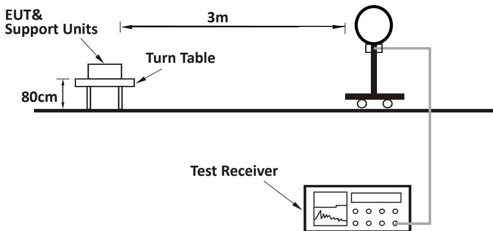
For Radiated emission 30MHz to 1GHz:
