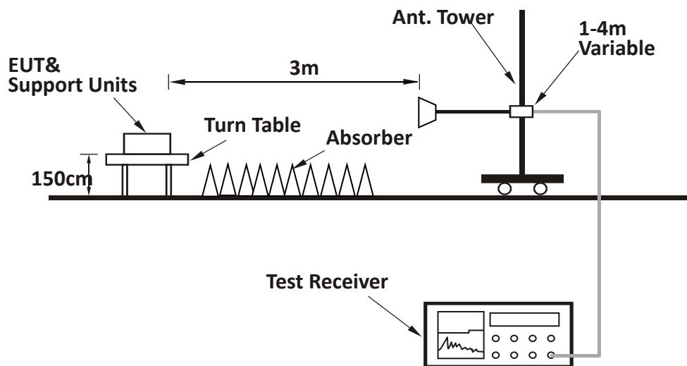
**TEST REPORT****7.4 Test Results of Radiated Emissions**
