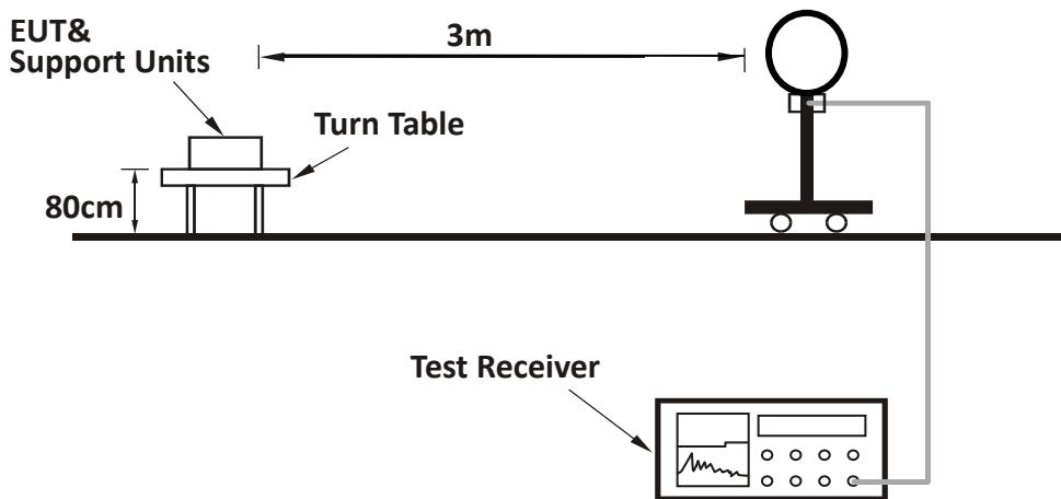
**For Radiated emission 30MHz to 1GHz:**
