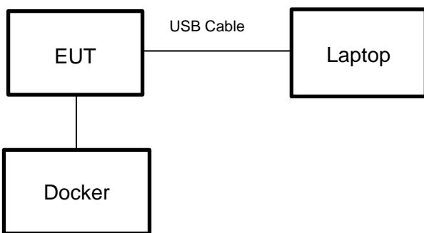
Note: The EUT can transmit independently and be charged with a docker. The docker is just a charger, not an intentional transmitter.
