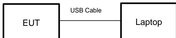
For Conducted Emission Test and Radiated Test:
