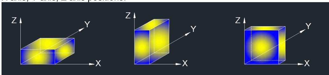
Note 1: For all radiated test, EUT in one orthogonal axis (X axis) emissions had been tested and recorded in the report.
