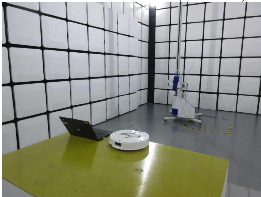
RADIATED RF MEASUREMENT SETUP (30MHz ~ 1 GHz)
