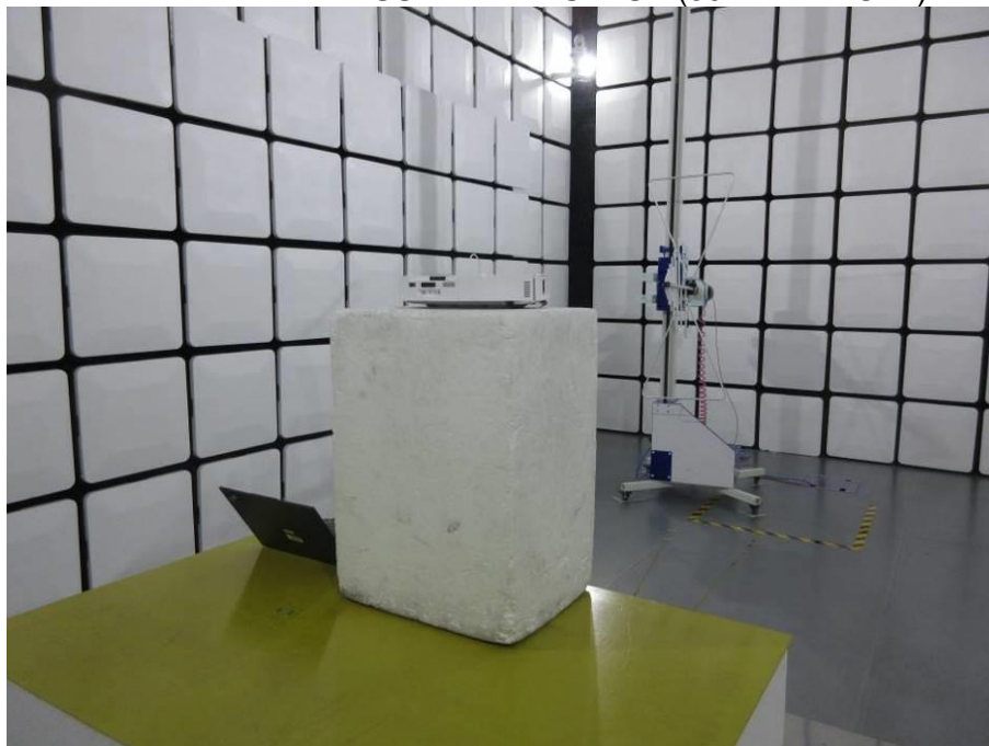
RADIATED RF MEASUREMENT SETUP (30MHz ~ 1 GHz)
