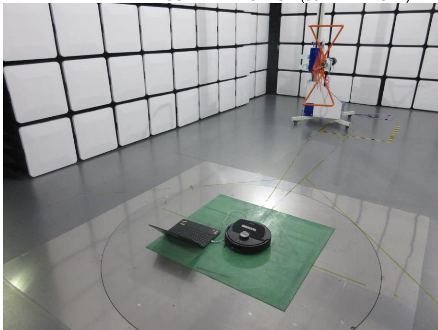
RADIATED RF MEASUREMENT SETUP (30MHz ~ 1 GHz)
