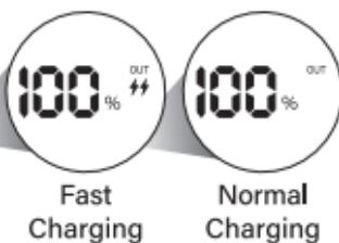
1. To charge compatible electronic devices with wired charging, connect it to the TYPE-C output port with the charging cable (not included) and do not press the button. (Lightning fast charging logo will appear after 10 seconds)
