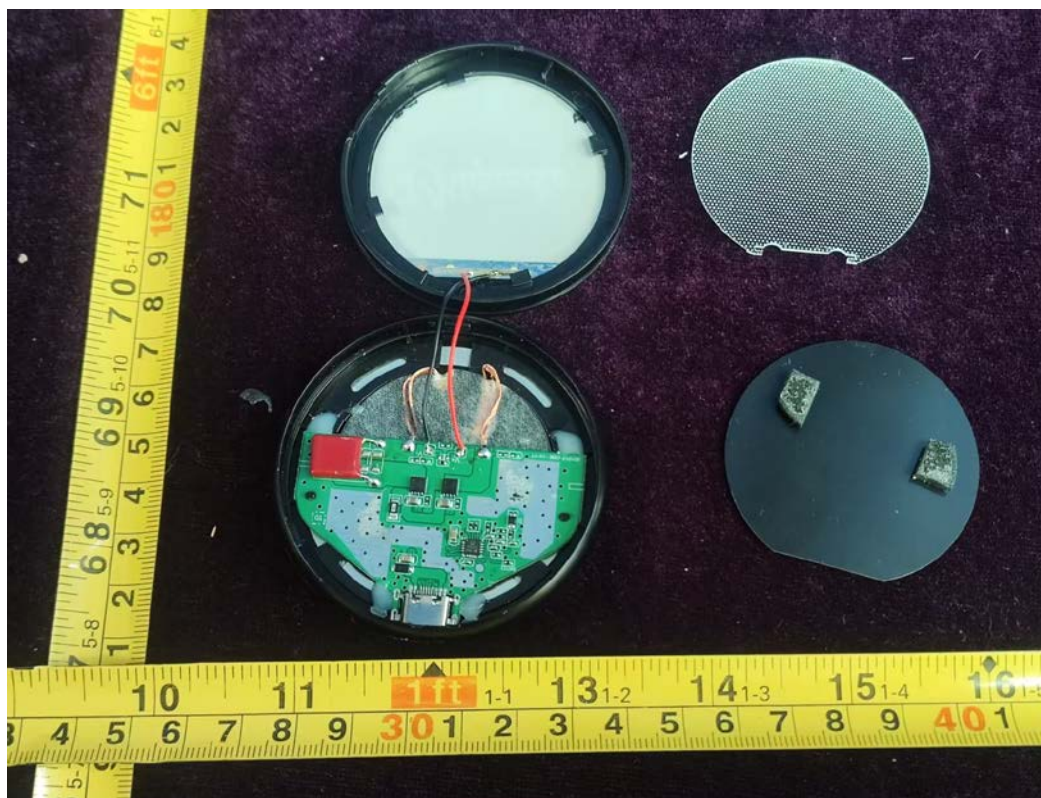
FIGURE 8 LIGHT UP MAGNETIC WIRELESS CHARGER (98371) MAINBOARD FRONT
