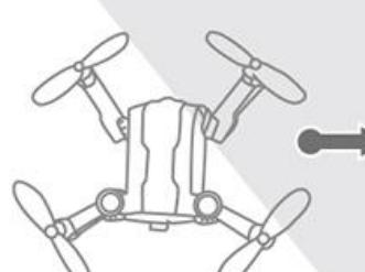
Slope the transmitter right and the drone will fly to the right.
