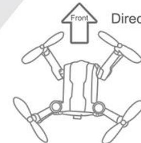
Press the headless mode button and the drone will enter headless mode.
