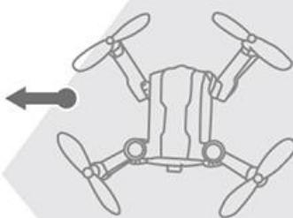
Slope the transmitter left and the drone will fly to the left.
