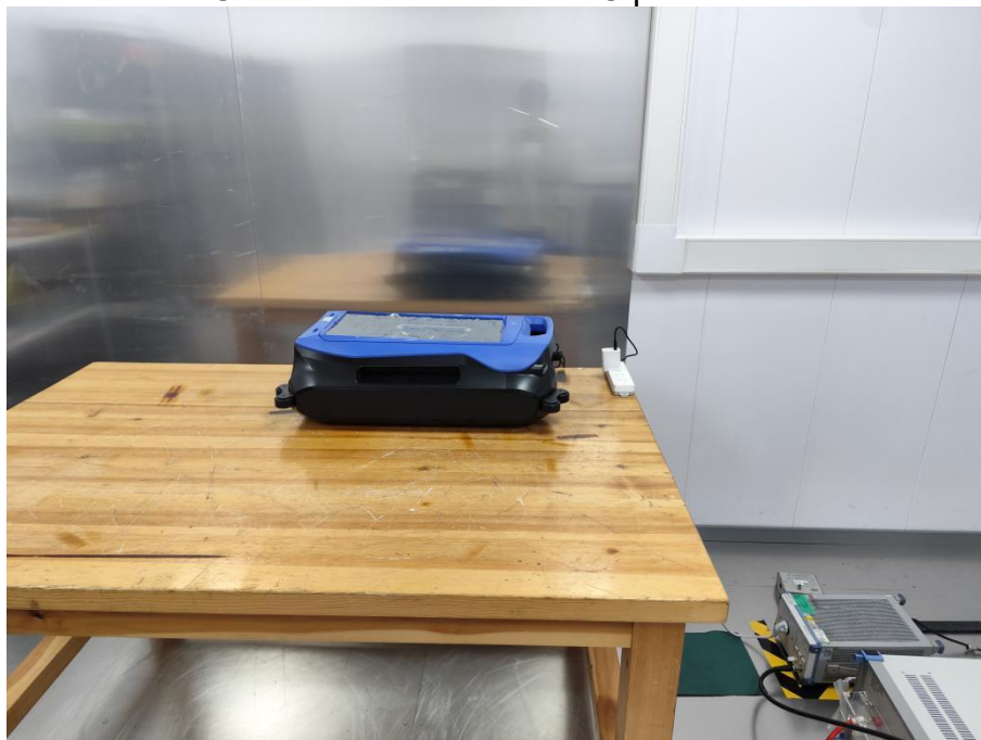
Conducted Emission at AC power line
