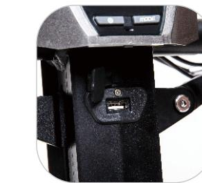
its built-in smart chip can provide 1-2A current output according to the need of charging equipment.
