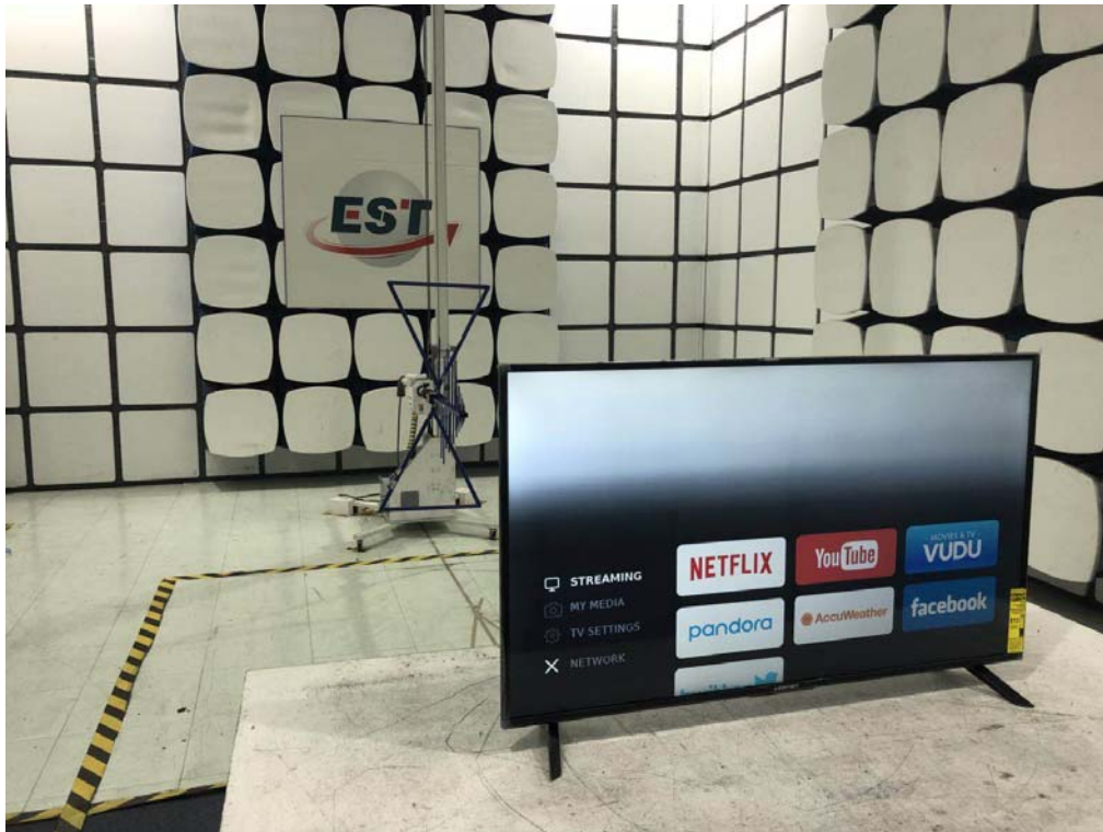
Radiated Test (30-1000 MHz)
