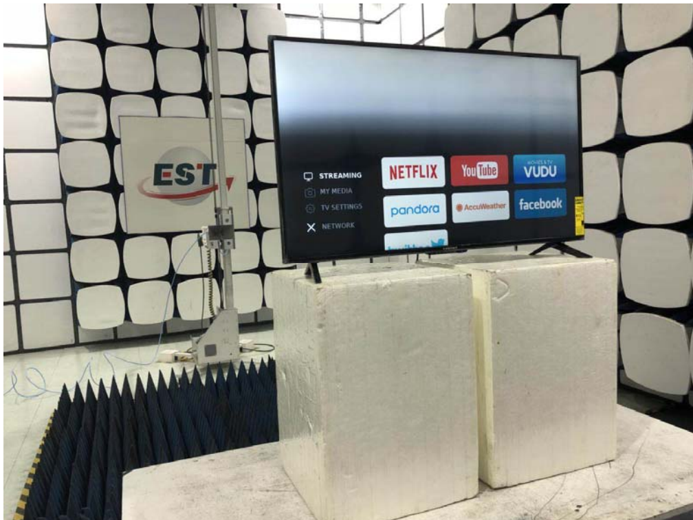
Radiated Test (Above 1GHz)
