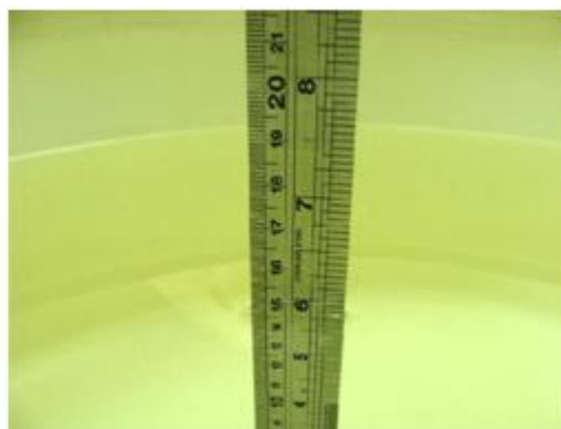
Fig 7.2 Photo of Liquid Height for Body SAR
