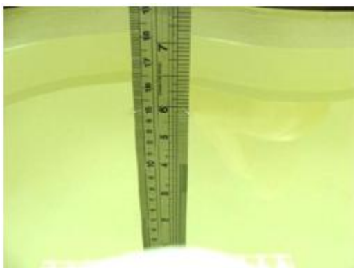
Fig 7.1 Photo of Liquid Height for Head SAR
