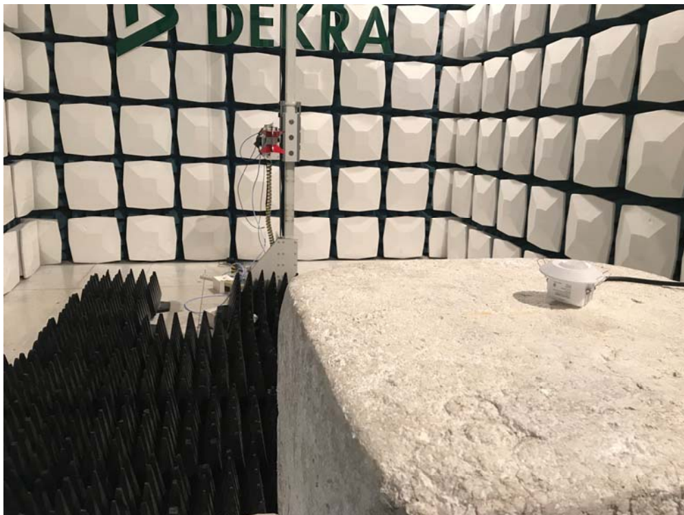
Description: Radiated Emission Test Setup for 1~18GHz
