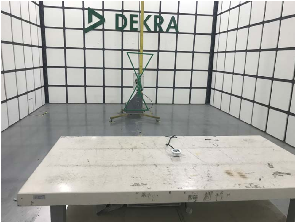
Description: Radiated Emission Test Setup for 1~18GHz
