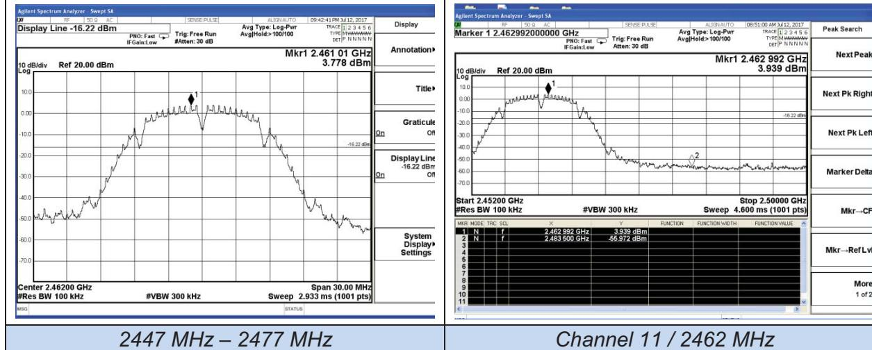
Band-edge measurements for conducted emissions
