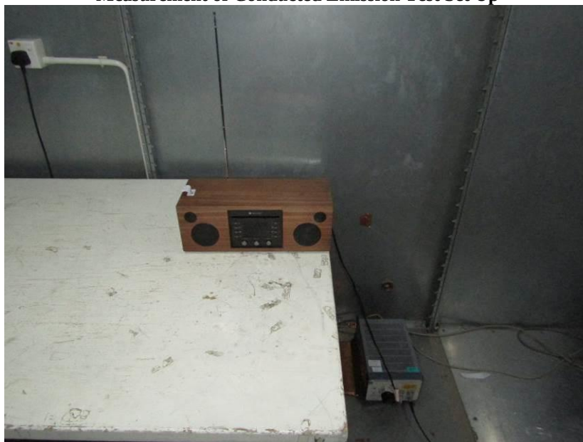
Measurement of Conducted Emission Test Set Up
