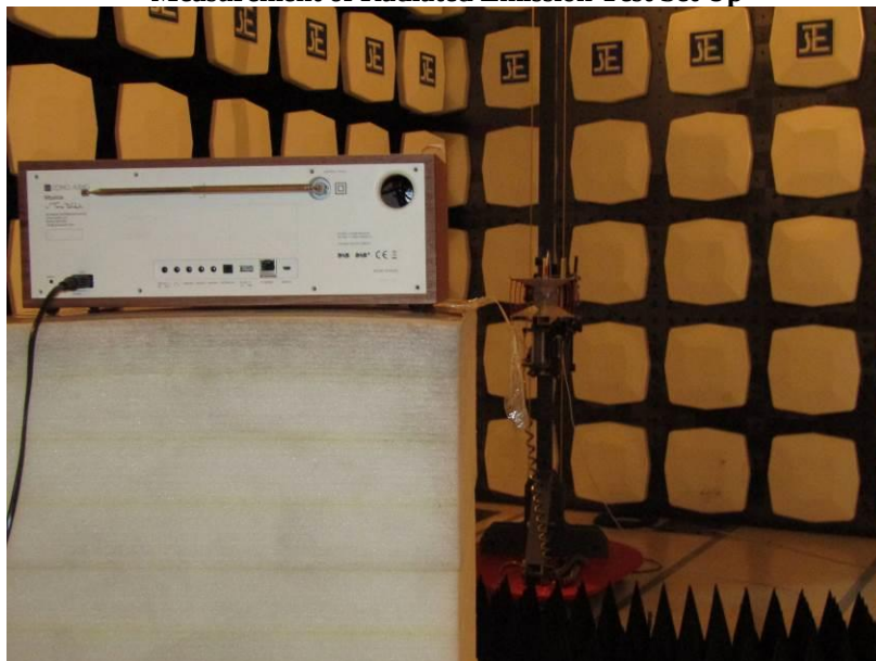
Measurement of Radiated Emission Test Set Up
