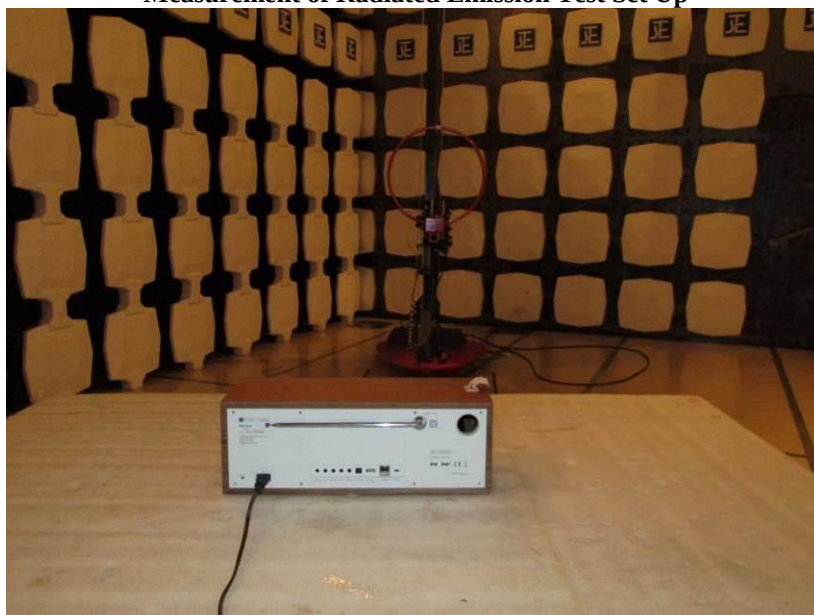
Measurement of Radiated Emission Test Set Up
