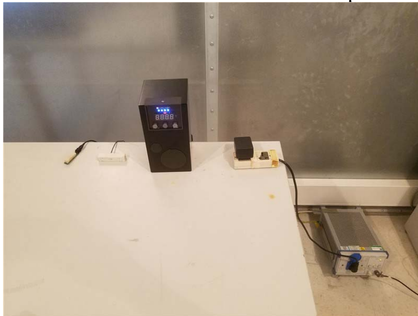
Measurement of Conducted Emission Test Set Up
