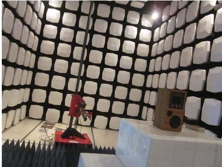
Measurement of Radiated Emission Test Set Up
