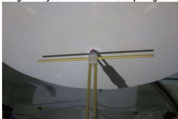
Fig.10.2 Photo of Dipole setup
