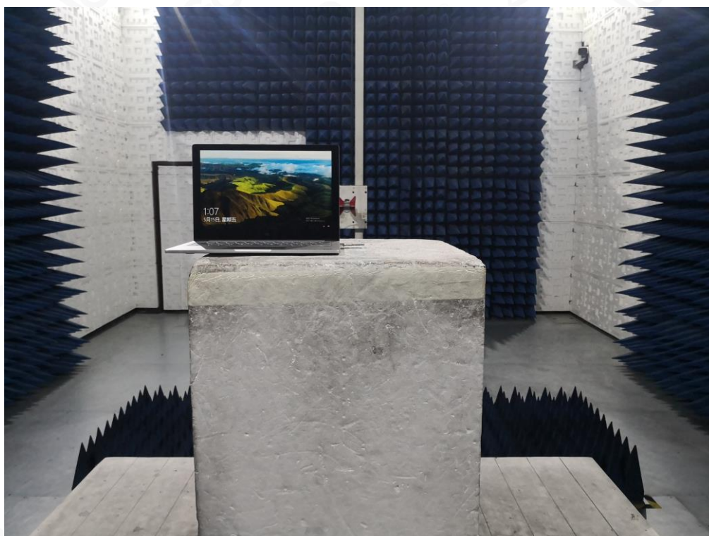
RADIATED EMISSION TEST SETUP ABOVE 1GHZ
