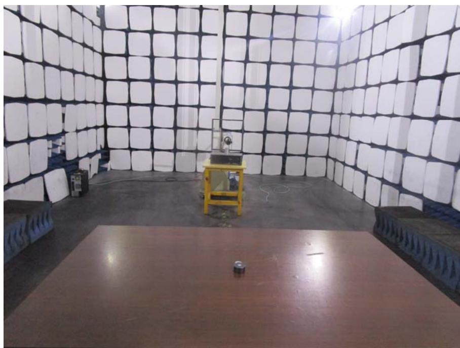
**Radiation Emission Test Setup (30MHz to 1GHz)**
