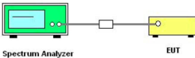
The EUT which is powered by the Battery, is coupled to the Spectrum Analyzer; the RF load attached to the EUT antenna terminal is 50 Ohm; the path loss as the factor is calibrated to correct the reading. Make the measurement with the spectrum analyzer's resolution bandwidth(RBW) = 100 kHz. In order to make an accurate measurement, set the span greater than RBW.
