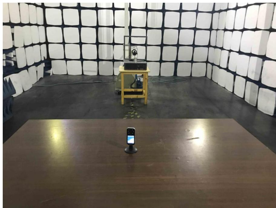
**Radiation Emission Test Setup (30MHz to 1GHz)**
