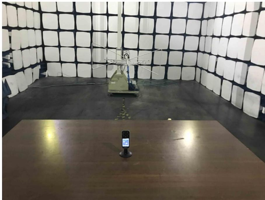
**Radiation Emission Test Setup (Above 1GHz)**
