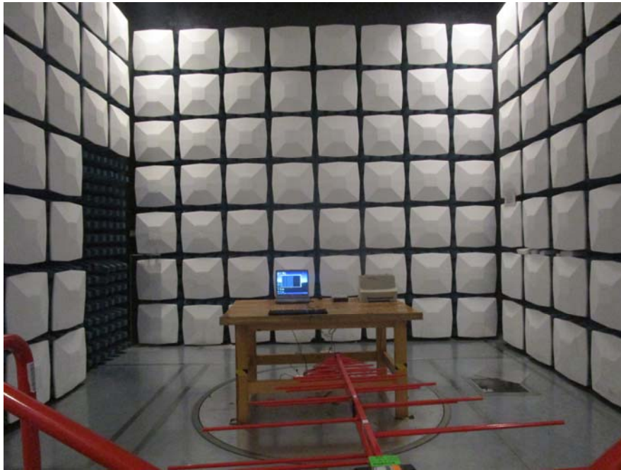
Radiated Emission Front View (Downloading Below 1GHz)
