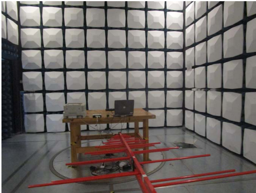
Radiated Emission Rear View (Downloading Below 1GHz)
