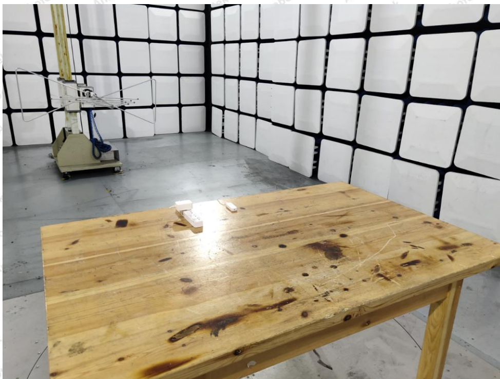
Photo of Radiation Emission Test
