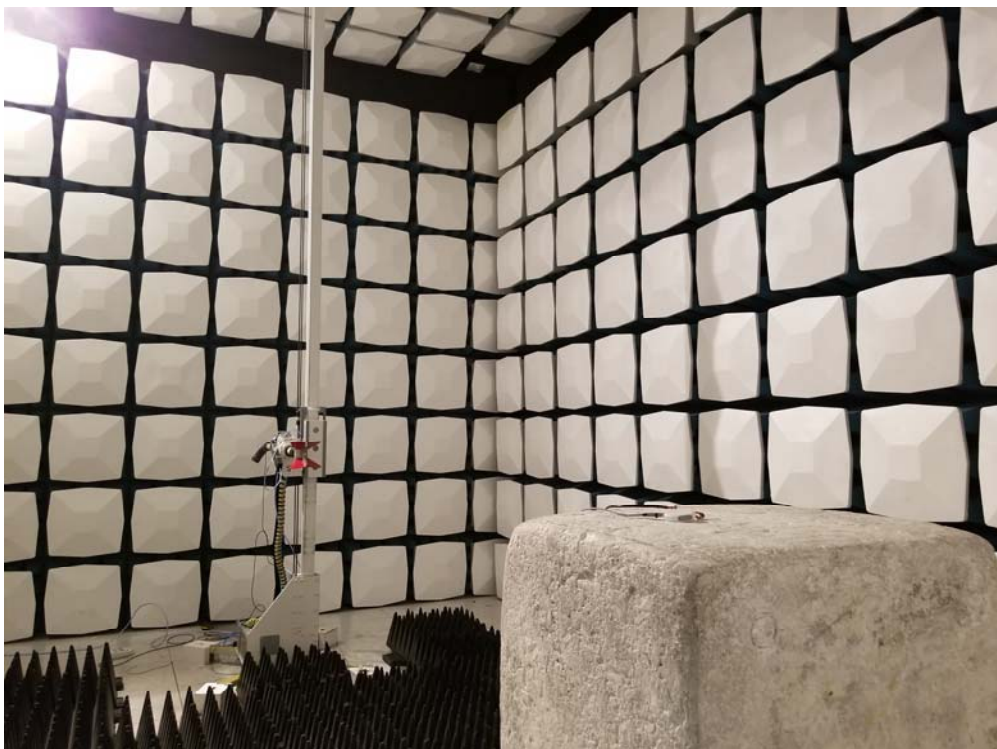
Description: Radiated Emission Test Setup for 1~18GHz
