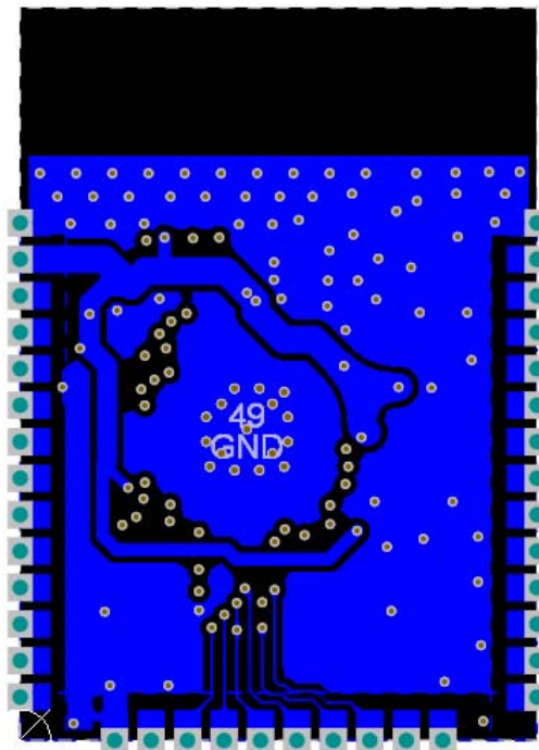
Figure 3 ESP32-S PCB POWER Layer
