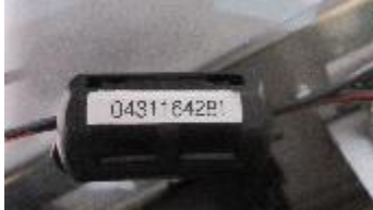
DC Power cable from switch to Control board ferrite PN 0431164281 one Loop
