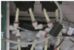
One Ferrite on Valve Cable Bundle near Control Board PN: 0461167281
