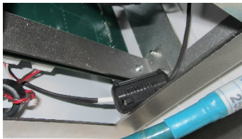
One Ferrite on LED Cable PN: 0431164281
