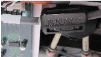
One Ferrite on Motor Cable bundle near Control Board PN: 0461167281
