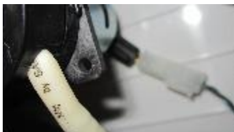
Pump 3 Cable at Pump Ferrite PN 046178181
