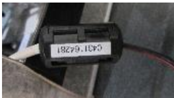
DC power from AC/DC Brick to switch/Fan Ferrite PN 0431164281
