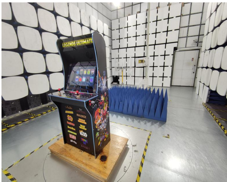
Photo of Radiated Measurement Above 1GHz
