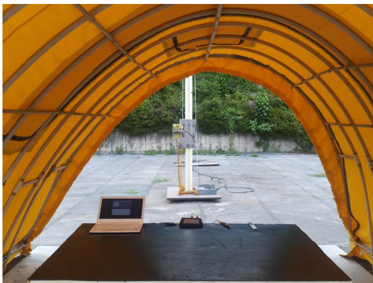
Photograph 2 : Setup for radiated Emissions (above 1 GHz)
