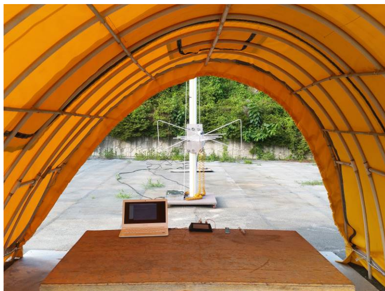
Photograph 1 : Setup for radiated Emissions (above 30 MHz)
